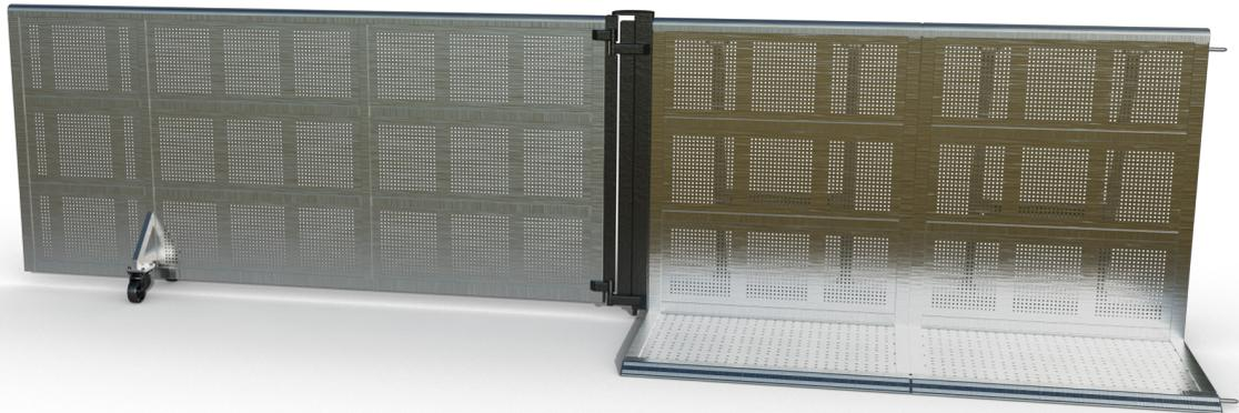
Dutch Barrier's Swing Gates come in left and right versions. This Right version opens to the right. Swing Gates are meant for emergency exits in low-pressure areas. There's no treadplate or lock, and they roll on wheels and, therefore, should always be manned by security personnel. One uses them in single or left-right configurations.
