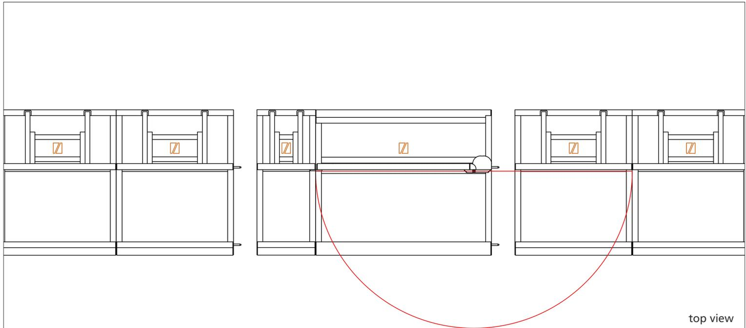
Testing was done at a minimum of 5kN/m pressure at the top rail, following and exceeding the Temporary Demountable Structures Edition 4 guidelines by the Institution of Structural Engineers (ISE). TUV reports for each test are available at Dutch Barrier & Dutch Barrier Services upon request.
