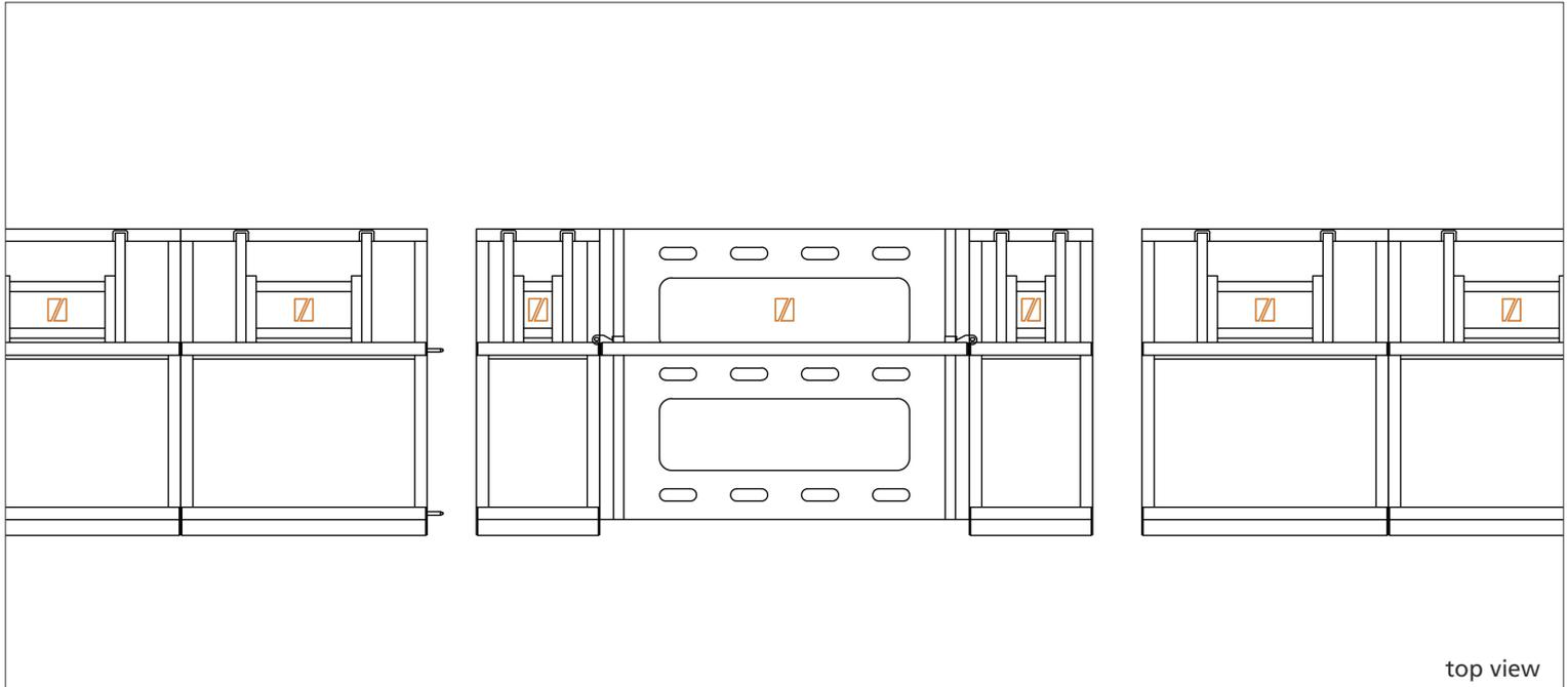
This unit will be tested at a minimum of 5kN/m pressure at the top rail, following and exceeding the Temporary Demountable Structures Edition 4 guidelines by the Institution of Structural Engineers (ISE). TUV reports for each test will be available at Dutch Barrier & Dutch Barrier Services upon request.
