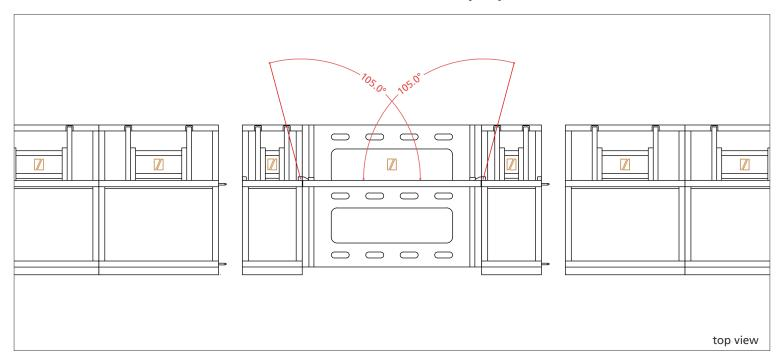
This unit will be tested at a minimum of 5kN/m pressure at the top rail, following and exceeding the Temporary Demountable Structures Edition 4 guidelines by the Institution of Structural Engineers (ISE). TUV reports for each test will be available at Dutch Barrier Services upon request.
